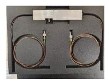
The product primarily completes the convention from electrical signals to optical signals, outputting in optical form for user applications. It mainly consists of an optical intensity modulator, a modulator driver control unit. The output optical interface of the product is in the form of an FC/APC connector, powered by an external power supply, and the component uses a non-sealed metal packaging.
